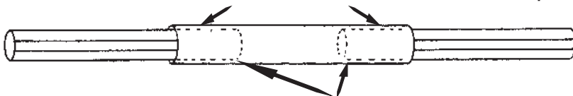
Fig. 2a Insert both end tubes equal distance into center tube and mark on center tube where inner tubes end
