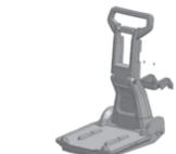
Insert Lower Hook using 2 self-tapping screws
