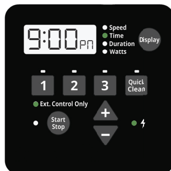
Figure 6: Activating External Control Only
