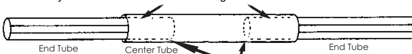
Fig. 3 Insert both End Tubes equal distance into Center Tube and Mark on Center Tube where inner tubes end.
