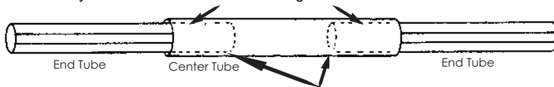
Fig. 3 Insert both End Tubes equal distance into Center Tube and Mark on Center Tube where inner tubes end.
