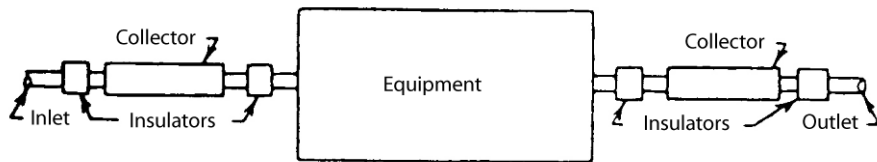
FIGURE 01. LEAKAGE CURRENT COLLECTOR DIAGRAM
