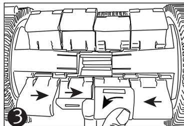
3 Once the inlet is removed you can remove any debris that is in the turbine chamber. You can also remove and replace the skirt/bracket assemblies. One of the middle skirt/brackets can be easily pulled out. Once one assembly is out you can slide the others out easily to replace.
